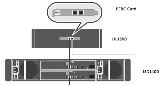
❑ **NOTE:** Turn on the system(s) only after setting up your DL Appliance hardware and connecting the DL Appliance to the optional MD1400 storage enclosure.
